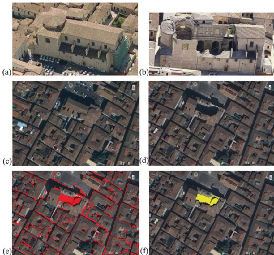
Fig. 8 The area around the church of Santa Maria Paganica: (a, c) Pre- and (b, d) post-event images. The comparison of classification shapefiles provide several errors shown in red colour (e), which are automatically filtered out with the removal of elongated features showing only shadows that indicated the damage, shown in yellow colour (f)
